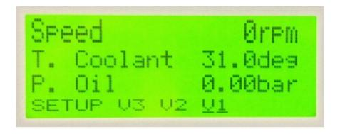
6) View screens can be manually programmed using the J1939 data by selecting values that begin with "EIC"
