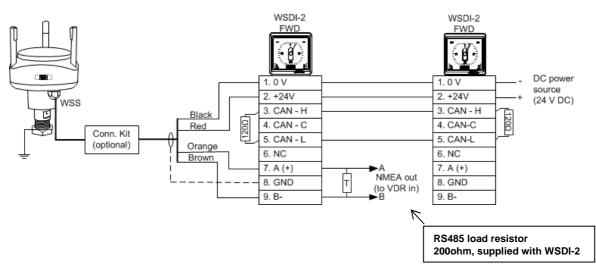
CANbus must be terminated in both ends.
