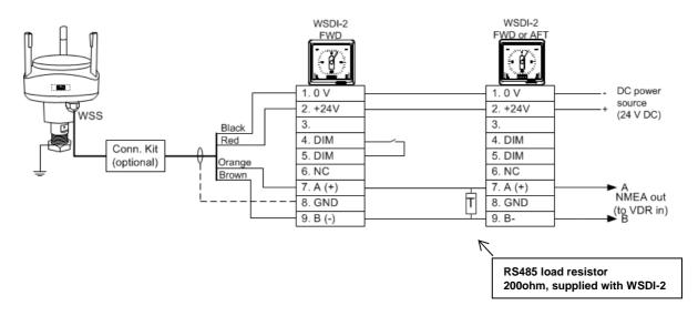
The WSS sensor can be connected to an extension cable using either the IP67 connector kit or IP66 connection box kit (optional accessories).
