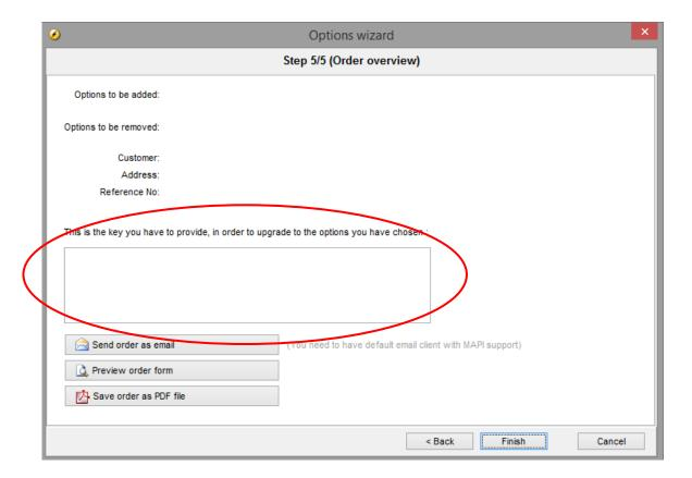
When receiving the option upgrade key simply click the "write new options" icon. Then copy and paste new key into field marked with red circle and press OK.
